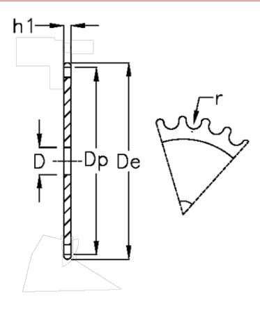
C = 6 D = 30 De = 474.2 Dp = 453.69 For chain size = 2 x 1 1/4 For chain type = 32 B-1 h1 = 29.4 Solution Number of teeth = 28
